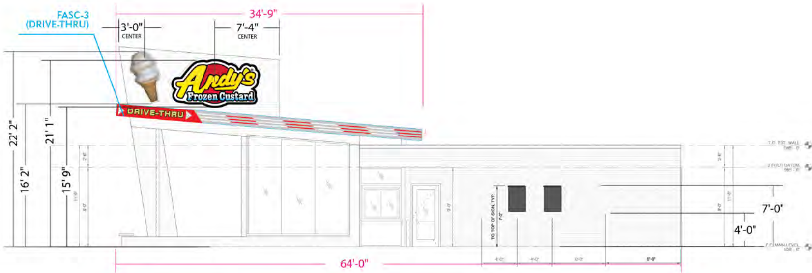
SIDE ELEVATION A - 64' LN. FT. / 73' SQ - EXTERIOR WALL SIGN / NEON = 58.5 sq ft / NON-ANIMATED
